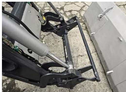
The operator can see the carriage during attachment by looking alongside the arms. The best approach, though, is to tip the frame completely.
