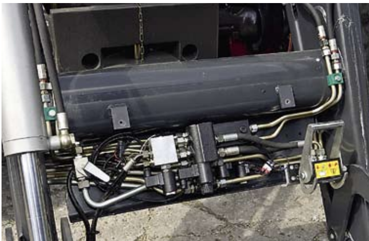
Attachment angle is shown by this telescopic rod, zeroed without having to resort to tools.
