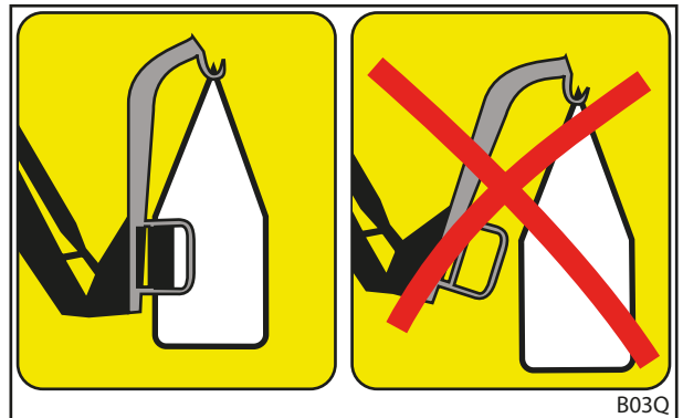
Fig. 79 Correct (left) and unsuitable position (right) of the implement
