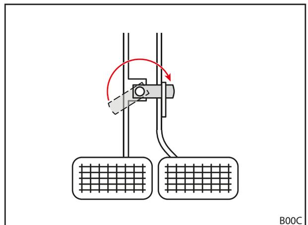
Fig. 43 Coupling the brake pedals
