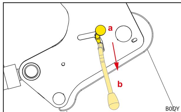
Fig. 55 Tensioning of the locking lever
