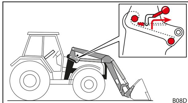
Fig. 122 Releasing the front loader locking mechanism
