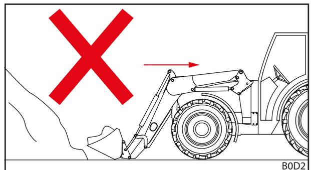
Fig. 111 Driving in reverse under load – Wrong
