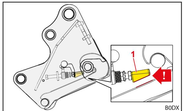
Fig. 52 Correct installation position of the clamping wedge
