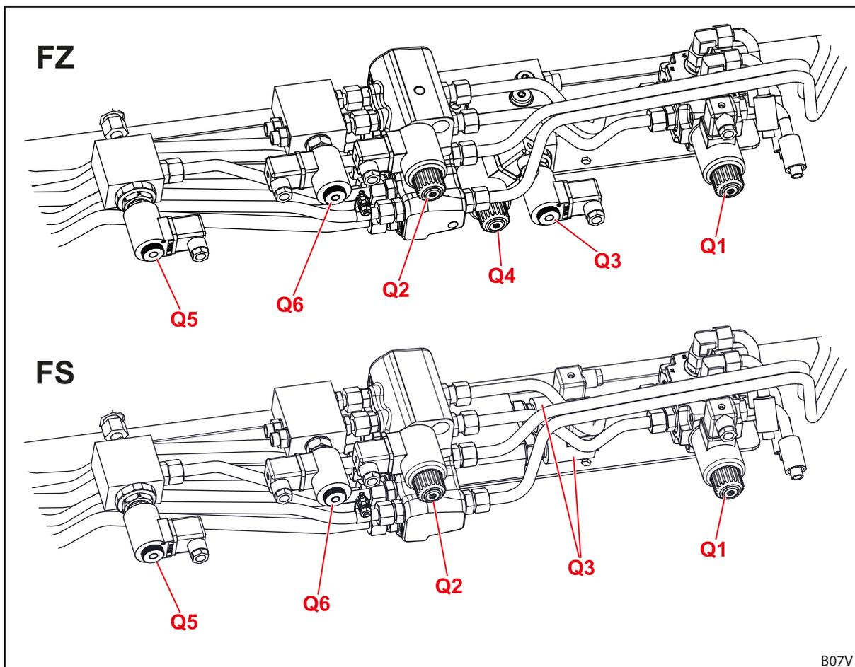
Fig. 133 Arrangement of the hydraulic valves for additional functions
