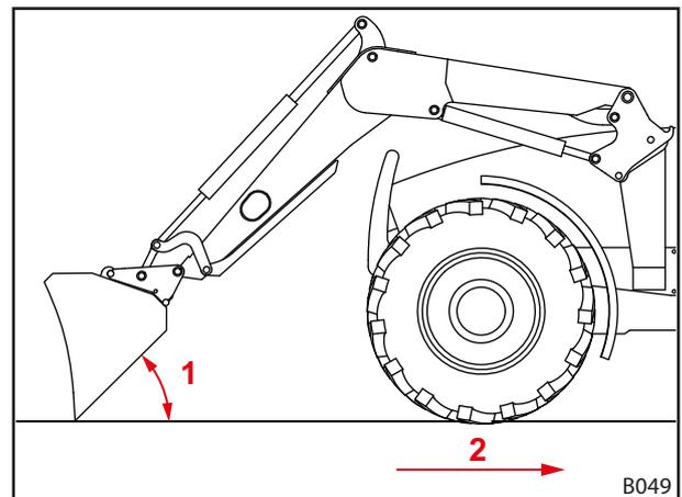
Fig. 108 Levelling in reverse
