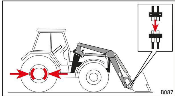
Fig. 97 Connecting the hydraulic lines of the implement to the front loader couplings
