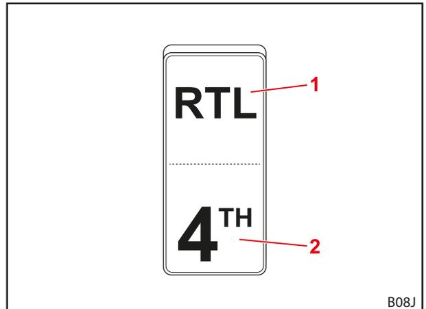
Fig. 71 Switch for the RTL function and 4th control circuit
