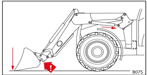
Fig. 84 Pressing the implement onto the ground
