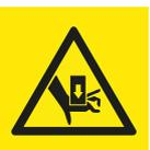
There is a risk of crushing of limbs when operating the parking supports to park the front loader, especially on uneven ground.
