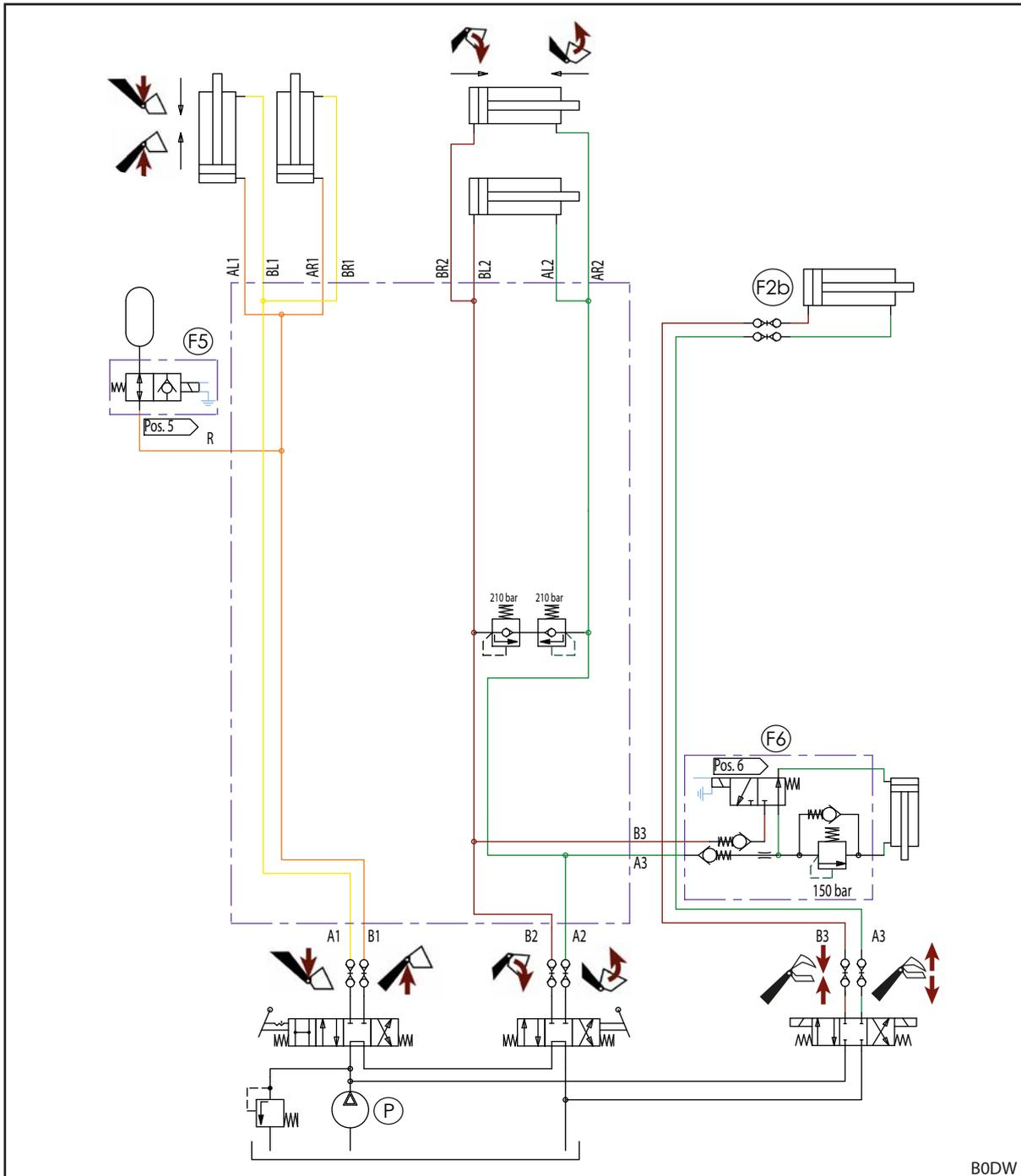
Fig. 128 FS hydraulic diagram (when equipped with REAL<sup>3</sup>)
