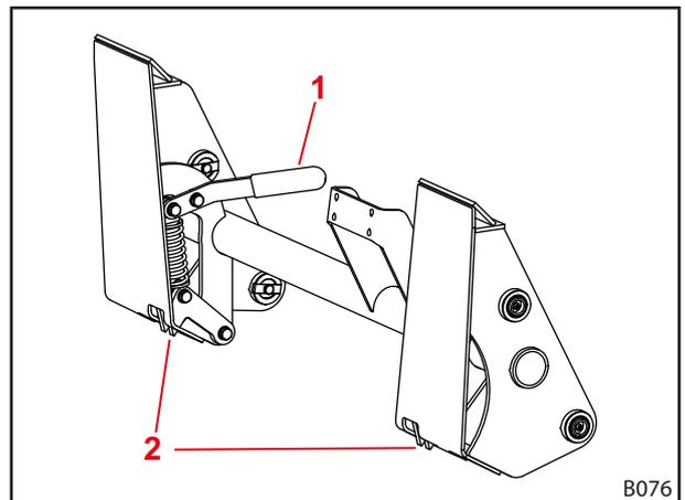
Fig. 85 Implement locking mechanism on skid-steer change frames
