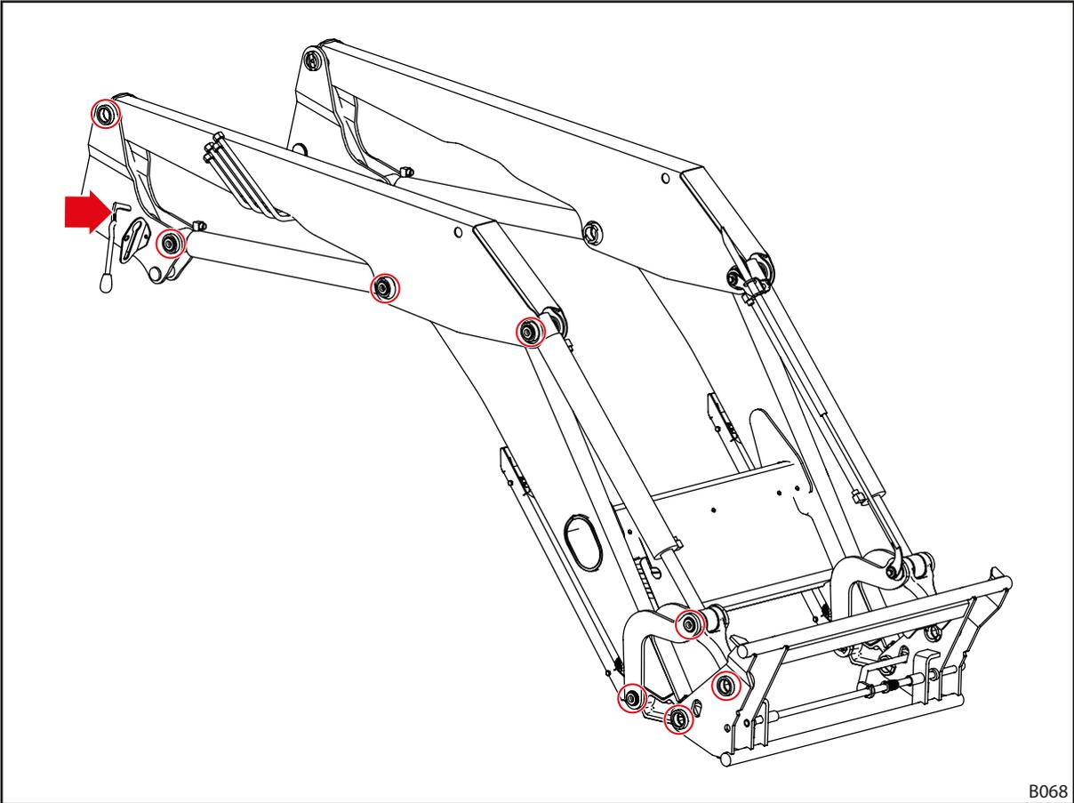
Fig. 114 Lubrication points on the FS
