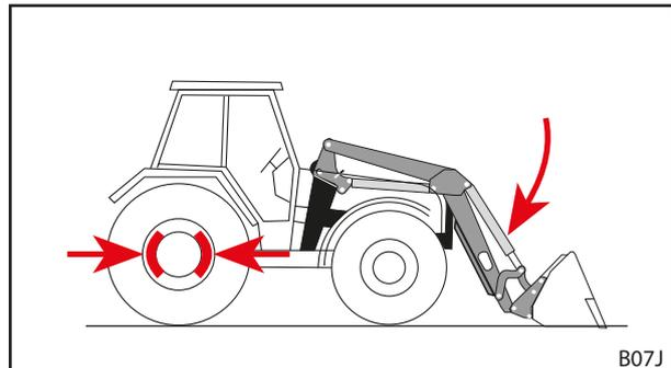
Fig. 121 Applying the parking brake and lowering the front loader
