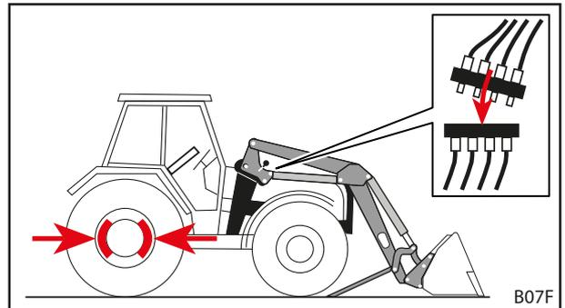
Fig. 49 Switching off the tractor and connecting the hydraulic lines
