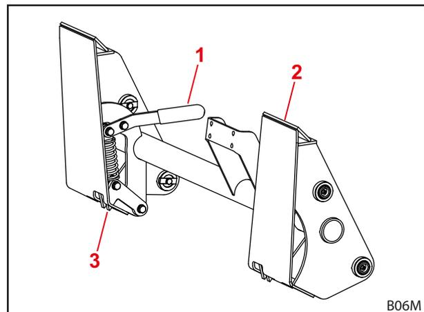
Fig. 26 Mechanical implement locking mechanism on skid-steer change frames
