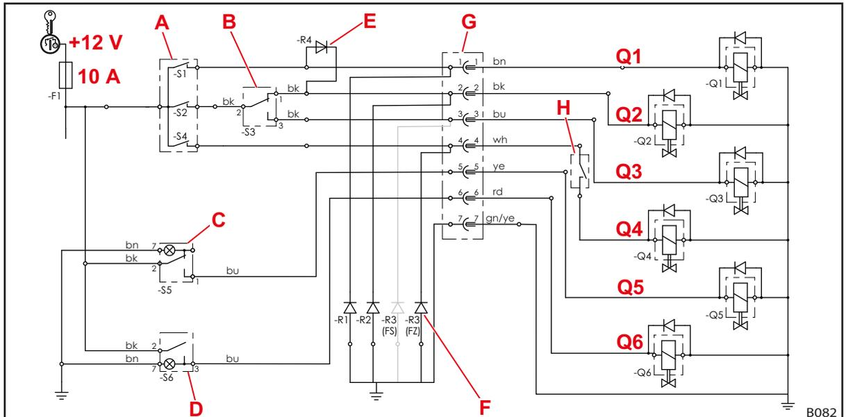
Fig. 131 Electric circuit diagram (when equipped with 3rd and 4th control circuit)
