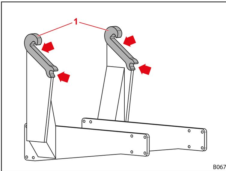
Fig. 113 Lubrication points on the front loader mountings
