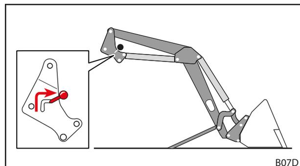
Fig. 47 Opening the front loader locking mechanism
