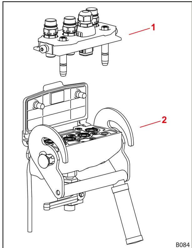
Fig. 22 Structure of the Hydro-Fix
