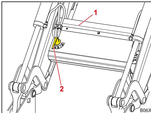
Fig. 40 Manually actuated Comfort Drive
