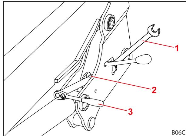
Fig. 54 Attaching the implement
