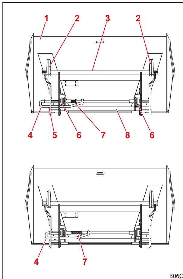
Fig. 25 Open (top) and closed (bottom) locking mechanism
