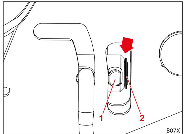
Fig. 119 Checking the gap
