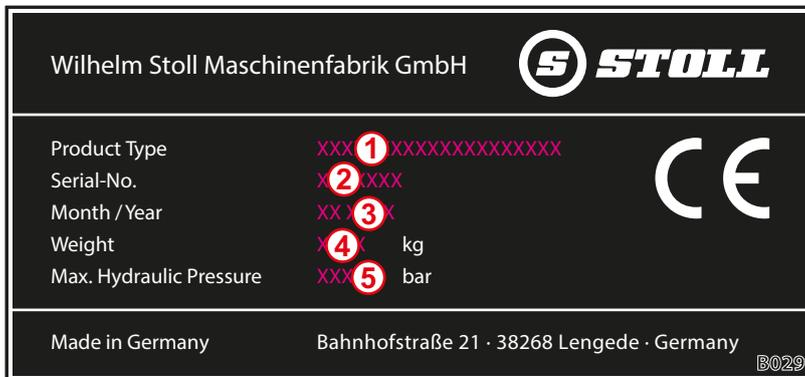
Fig. 1 Rating plate on the front loader
