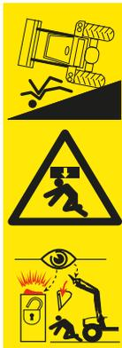
There is a risk of serious injury and mortal danger when loading and transporting loads, if the front loader is operated from one side, the load is raised too far over the driver's seat or if unsuitable implements are used.
