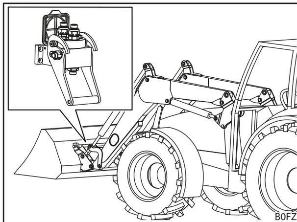
Fig. 23 Implement-Fix: position on the front loader
