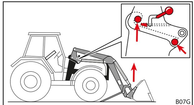
Fig. 50 Using the lifting function until the front loader pins are resting in the catch hooks
