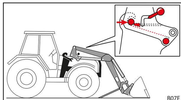
Fig. 48 Driving the tractor into the lifting arm
