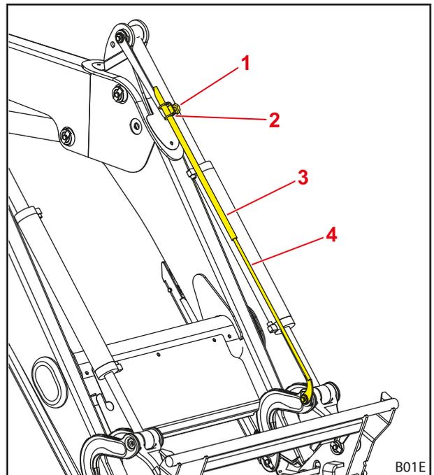
Fig. 32 Indicator for implement position
