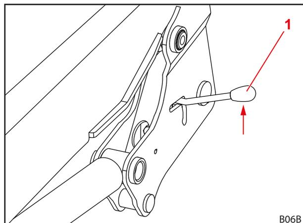
Fig. 117 Checking the front loader locking mechanism
