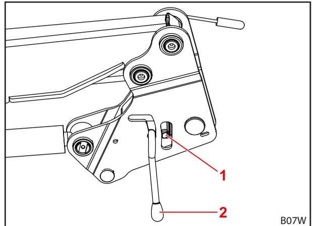
Fig. 118 Checking the front loader locking mechanism
