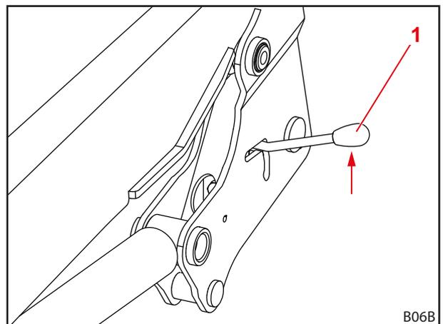
Fig. 53 Opening the front loader locking mechanism
