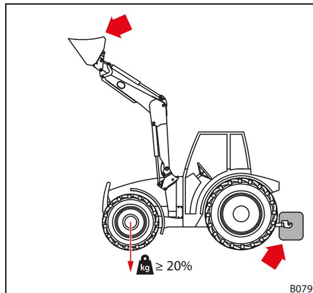
Fig. 45 Load for driving on roads
