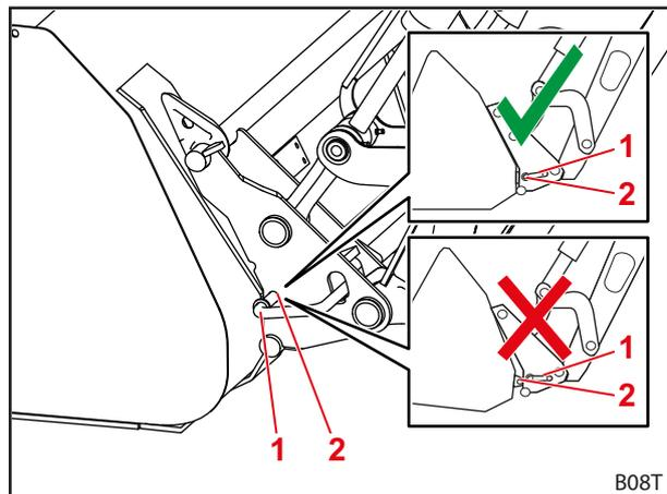
Fig. 83 Checking the position of the locking pins
