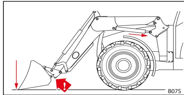
Fig. 91 Pressing the implement onto the ground
