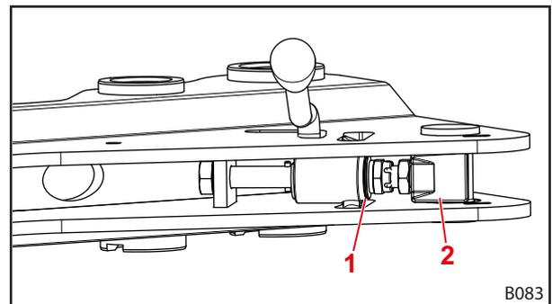
Fig. 60 View of the front loader locking mechanism from below
