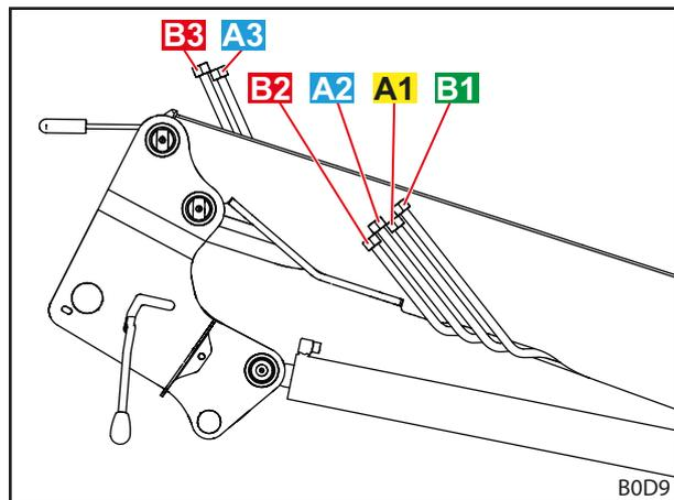
Fig. 18 Hydraulic lines (REAL<sup>3</sup> option)
