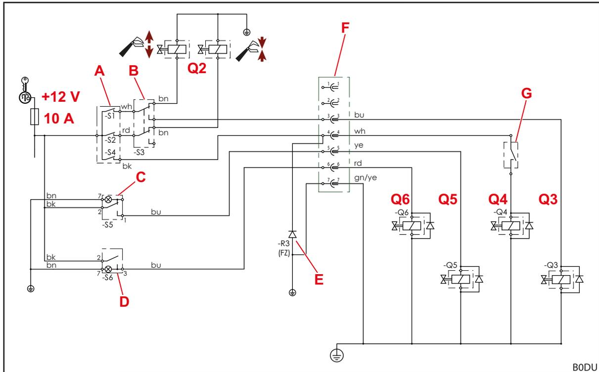
Fig. 132 Electric circuit diagram (when equipped with REAL<sup>3</sup>)
