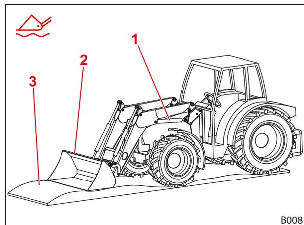
Fig. 31 Front loader in float position
