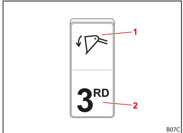
Fig. 70 Switch for rapid or quick emptying and 3rd control circuit or REAL<sup>3</sup>
