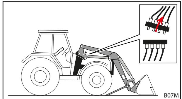
Fig. 124 Uncoupling the hydraulic system
