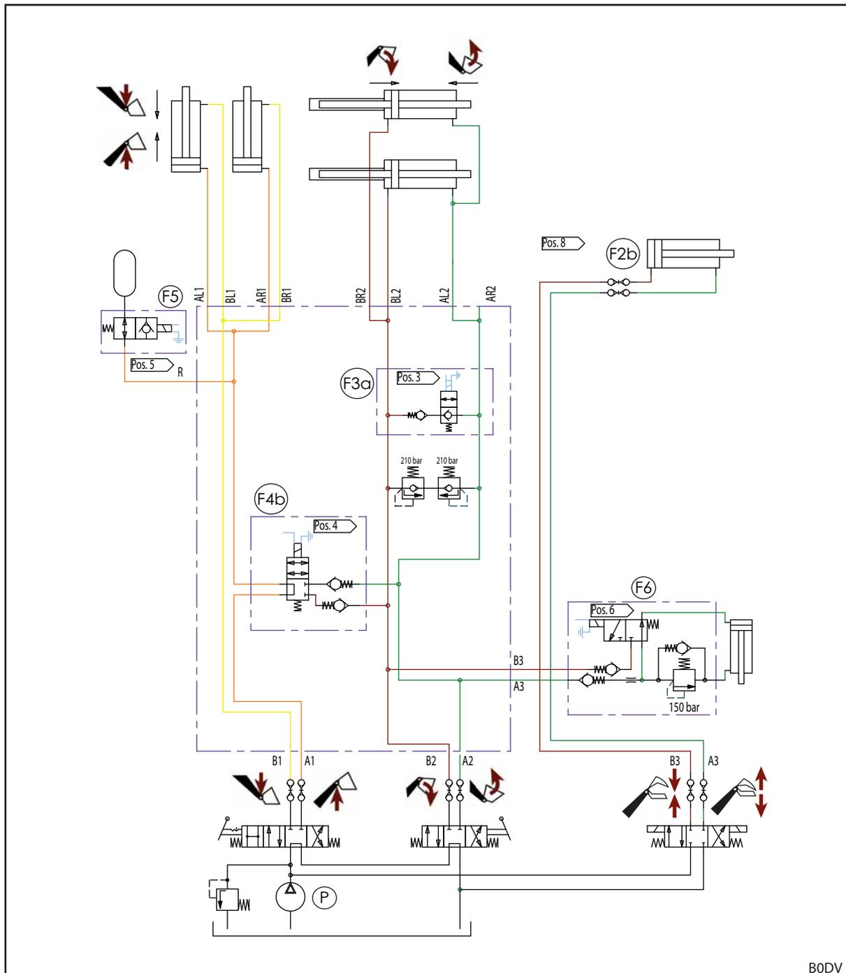
Fig. 130 FZ and FZ-L hydraulic diagram (when equipped with REAL<sup>3</sup>)
