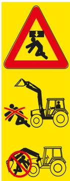
There is a lethal risk of crushing and injury due to accidental movements of the tractor, the front loader, and the implements.
