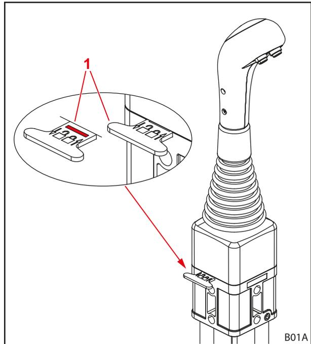
Fig. 65 Locking the operating lever
