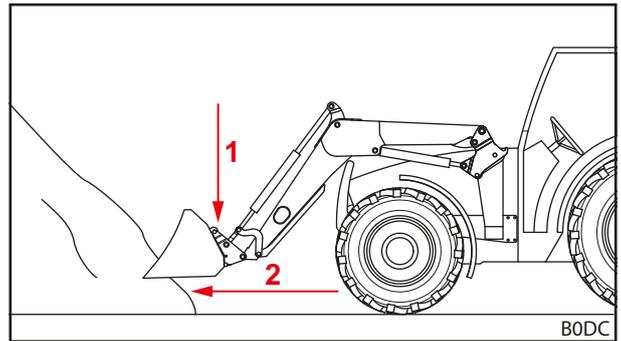
Fig. 109 Lowering the front loader and driving straight into the load
