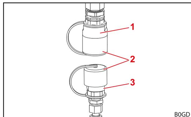
Fig. 76 Screw couplings (sample illustration)
