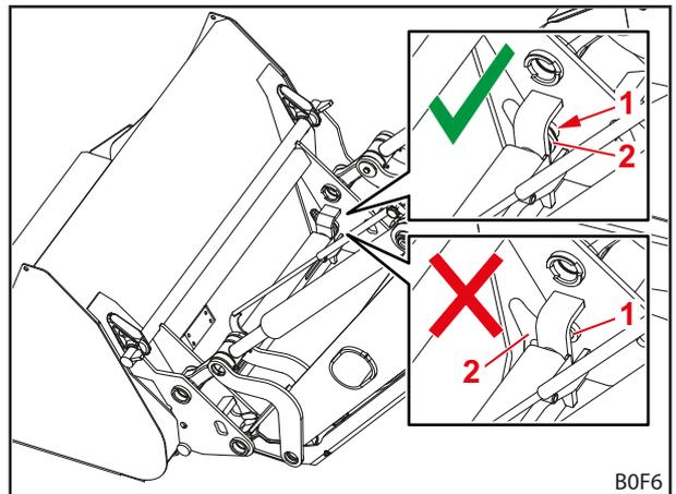
Fig. 90 Checking the position of the locking pins
