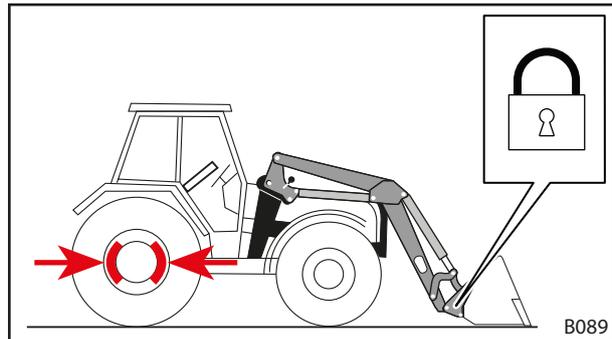
Fig. 101 Closing the implement locking mechanism
