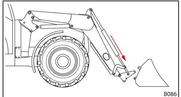
Fig. 93 Position the lifting arm
