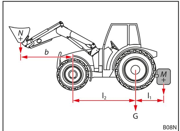
Fig. 46 Calculation of the static stability
