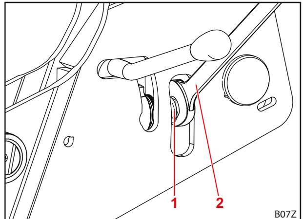
Fig. 58 Attaching the implement
