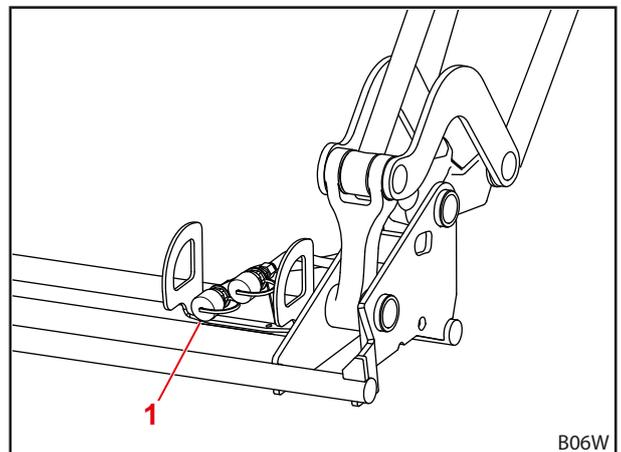
Fig. 37 Additional 3rd control circuit
