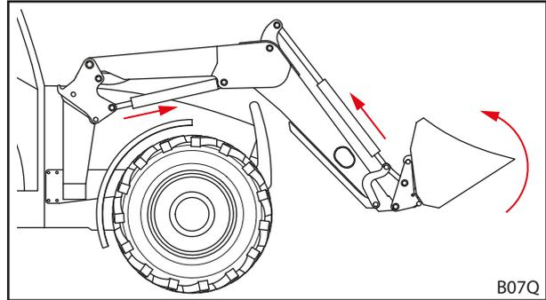
Fig. 96 Triggering the implement locking mechanism
