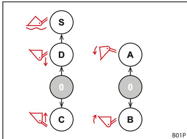
Fig. 63 Assignment with 2 operating levers
