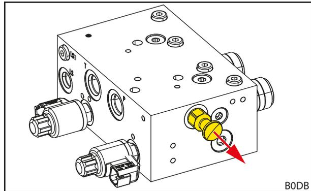
Fig. 72 Pulling out the pressure relief valve on the REAL<sup>3</sup> valve
