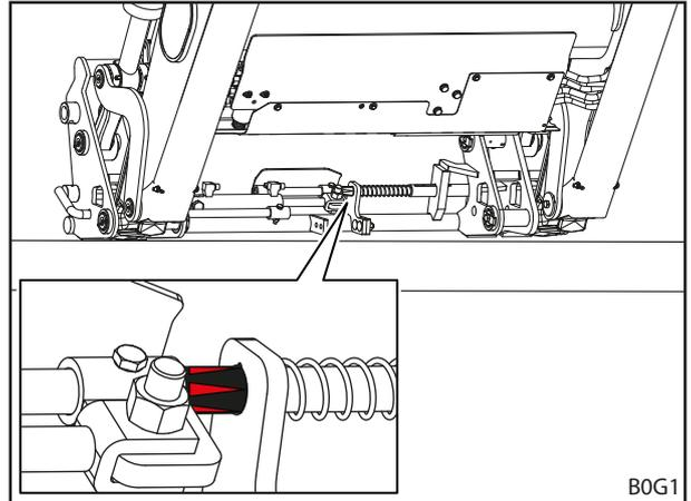
Fig. 88 Using the sticker to check the implement locking mechanism
