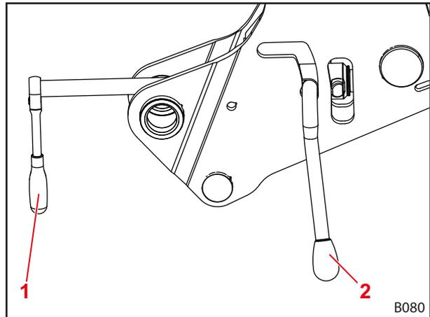
Fig. 59 Guiding the socket wrench through to the screw
