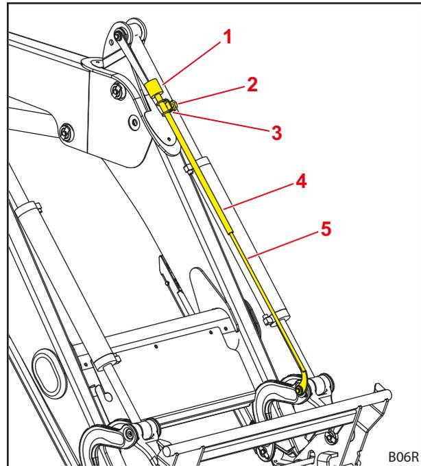
Fig. 36 Return To Level sensor on the indicator
