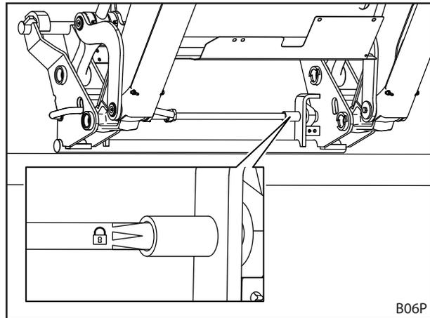
Fig. 81 Using the sticker to check the implement locking mechanism
