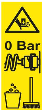
There is a risk of crushing when machine parts move uncontrollably due to entrapped air in the hydraulic system.
