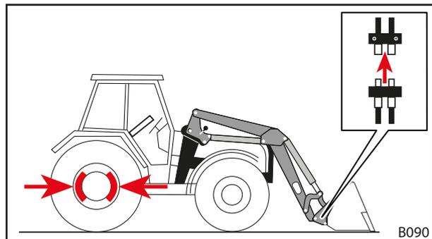
Fig. 105 Releasing the hydraulic lines
