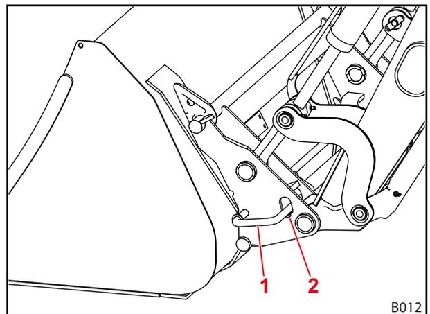
Fig. 80 Mechanical implement locking mechanism
