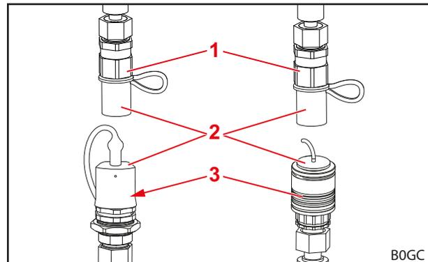
Fig. 75 Plug-in couplings (sample illustrations)
