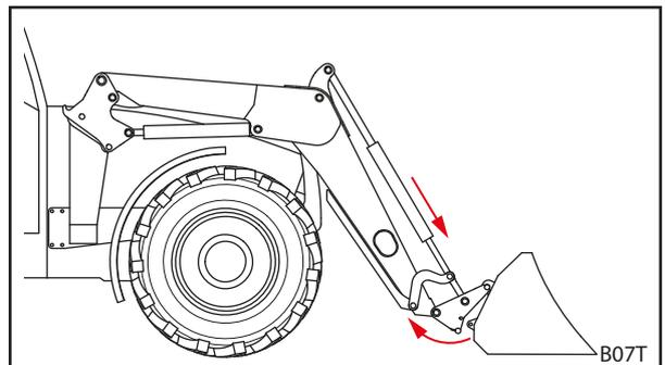
Fig. 106 Unhooking the change frame
