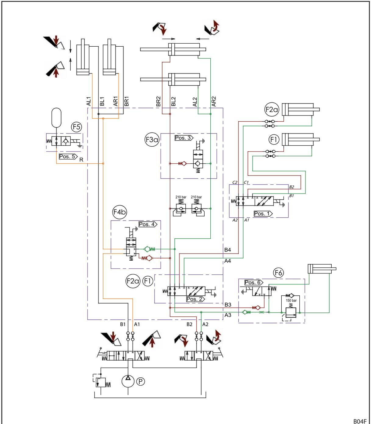
Fig. 129 FZ and FZ-L hydraulic diagram (when equipped with 3rd and 4th control circuit)
