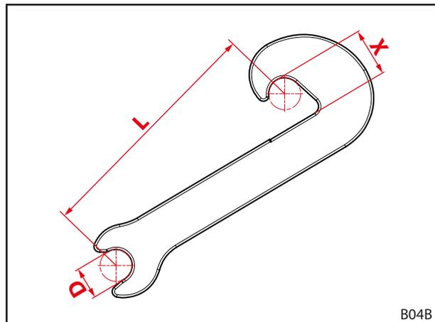
Fig. 116 Wear dimensions of the catch hook
