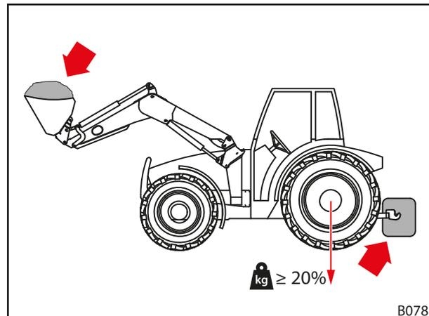
Fig. 44 Load for front loader work
