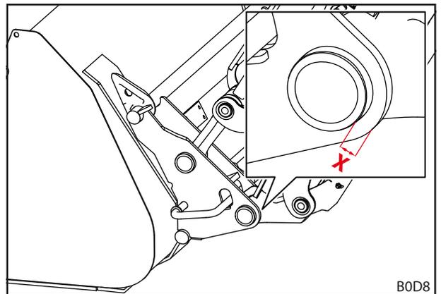
Fig. 120 Wear dimension of the change frame
