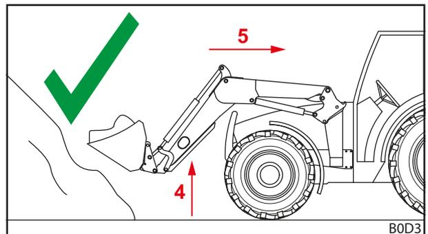
Fig. 112 Driving in reverse under load – Right
