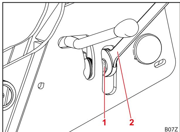
Fig. 61 Tightening the locknut
