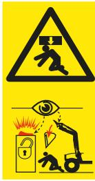
There is a risk of serious injury and lethal danger due to implements falling down or uncontrolled lowering of the front loader when unsuitable implements are used or if the used implements are overloaded.
