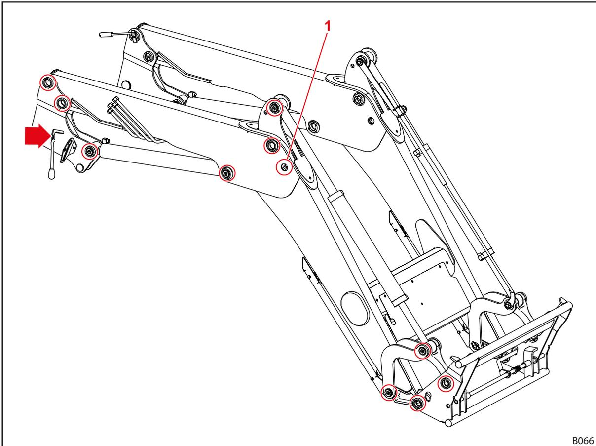
Fig. 115 Lubrication points on the FZ
