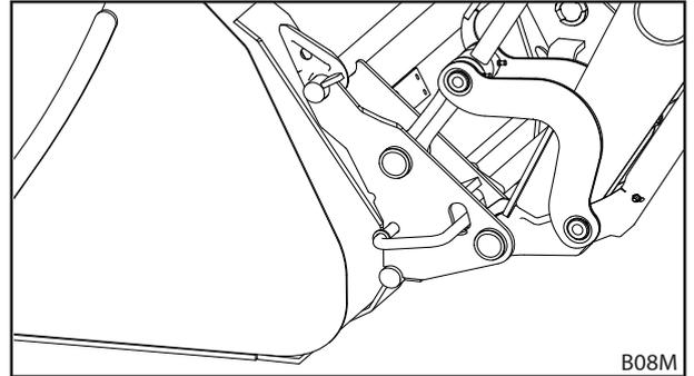
Fig. 92 Opening the implement locking mechanism
