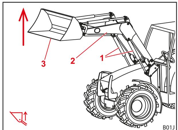
Fig. 27 Lifting function
