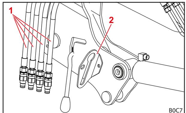
Fig. 126 Hanging the hydraulic lines on the coupling mount (shown with plug-in couplings)
