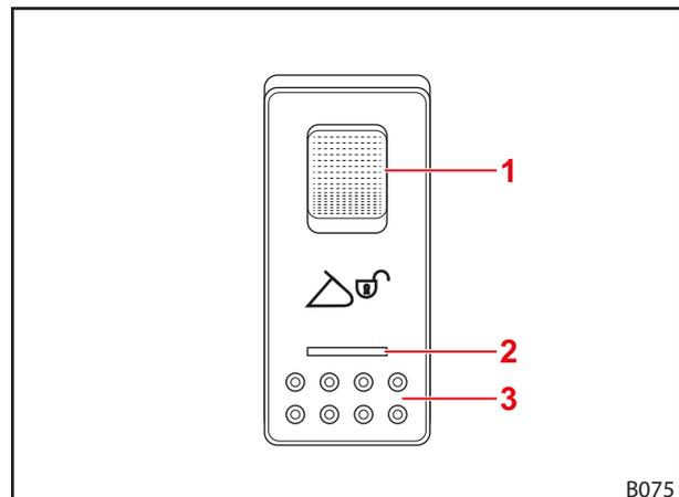
Fig. 87 Hydro-Lock switch
