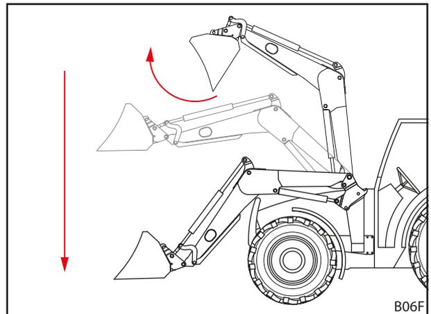
Fig. 35 Return To Level function
