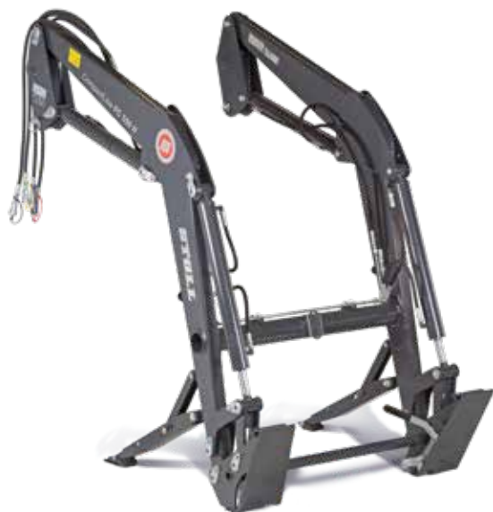
FC-H lifting arms without parallel linkage
