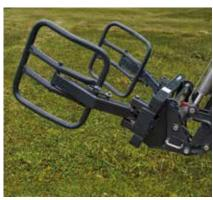
Tilt the implement – the locking mechanism automatically slots into place.
