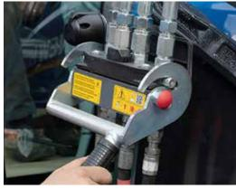
With the Hydro-Fix all hydraulic lines can be connected to the tractor at the same time. The front loader is lifted slightly to hold the locking pin in position in the catch hook of the connection support.
