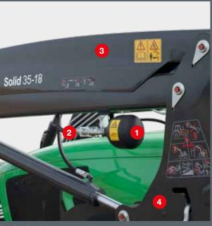
The Comfort-Drive is protected between the drive-in column and the lifting arm bar. It can be switched on and off with the stopcock.
