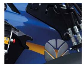
When driving in, the front loader slides along the attachment component until the locking pin meets the upper end of the connection support.
