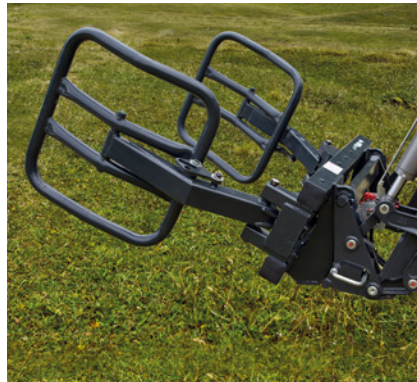
2 Tilt the implement – the locking mechanism automatically slots into place.
