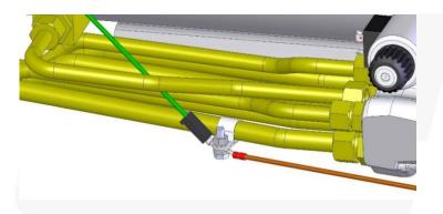
With the Pro Control controls, the grounding connection is integrated in the wiring harness and is an important component of the system's automatic supervision. This line is needed, for example, to identify short circuits or cable breaks in the system and to deactivate specific functions in the case of any faults.
