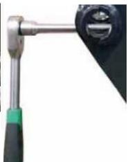
To set the lock, you will need an open-ended spanner (WAF 30), a ½" ratchet with the corresponding extension and 30 mm socket spanner.
