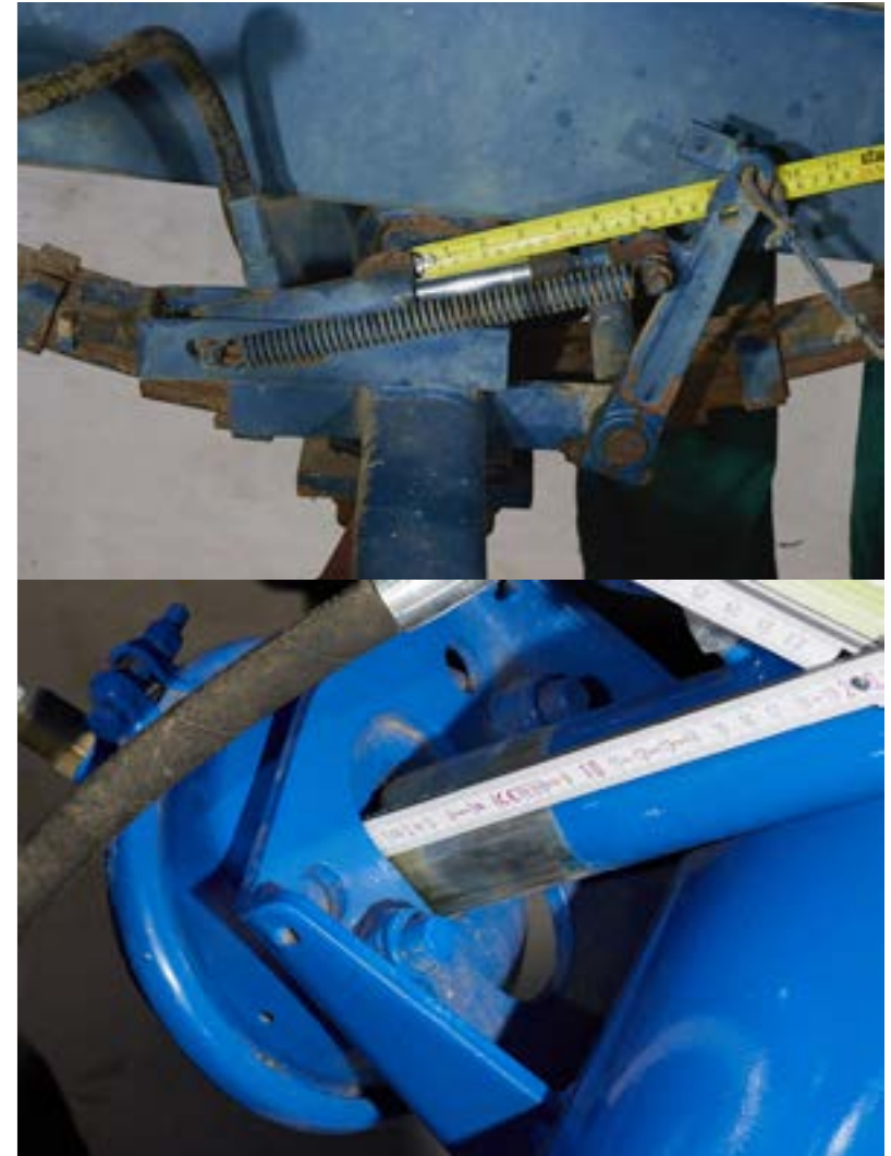
Fig.17 Excessive brake actuator free travel = No Brakes!
