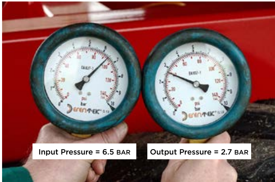
Fig.26 Load Sensing Valve (LSV) input and output pressure levels for an example unladen trailer
