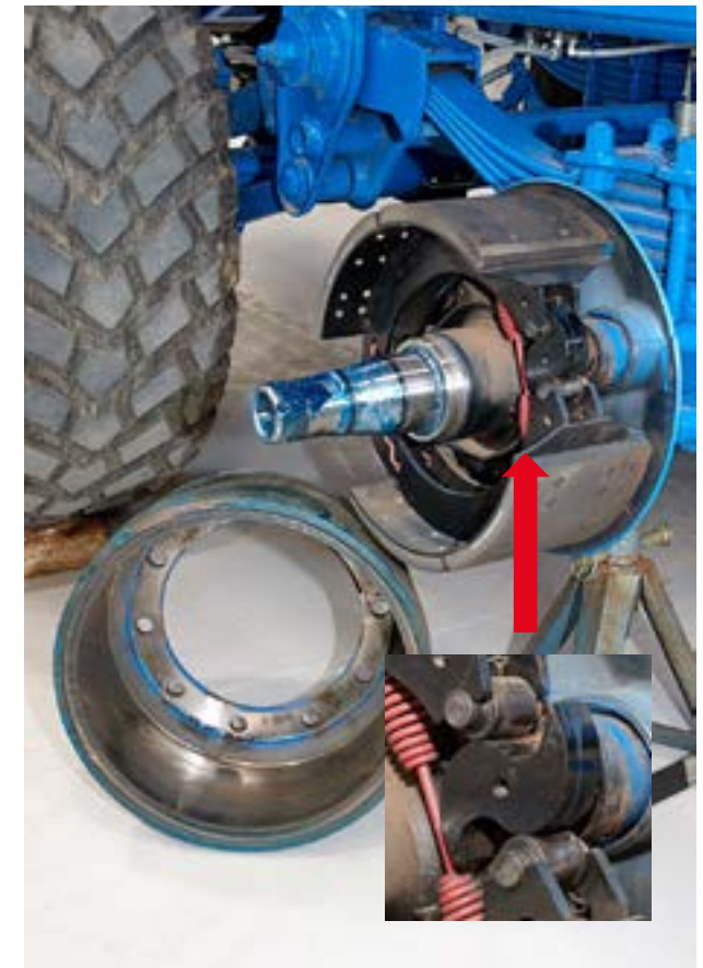
Fig.14 Example Commercial 'High-Speed' brake and drum- Note 'S'-type operating cam (arrowed & inset)
