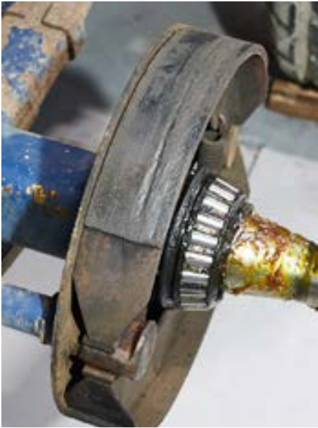
Fig.29 Damaged/overheated trailer brake friction lining
