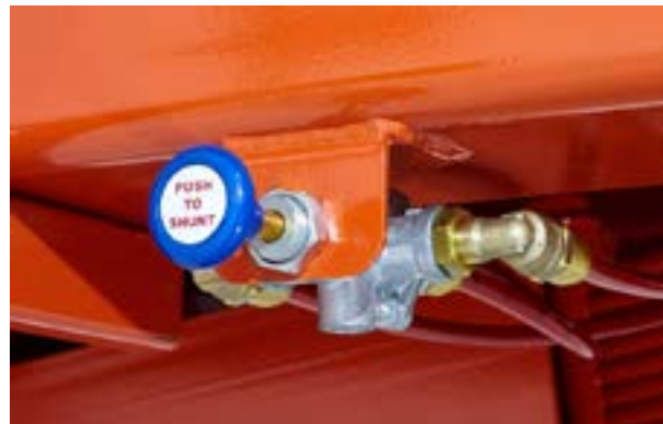
Fig.10 Shunt valve fitted to an air-braked trailer
