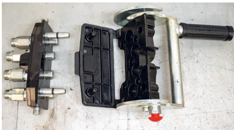
Retrofit quick couplers will cost around £515 but check as different couplings may be needed for some older loaders. These couplings allow coupling under pressure.
