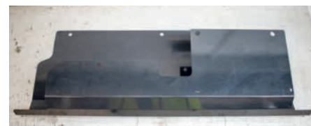
The hose protection plate under the cross beam can get bent or removed and lost. A new cross plate is £100.
