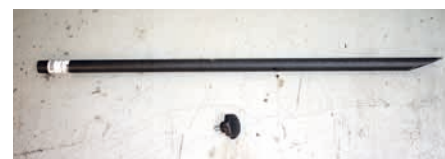
The simple rod level indicator adjusts to suit different attachments. It can get damaged or the lock nut adjuster wind off and get lost. A new tube is £30, the knob £3.00.
