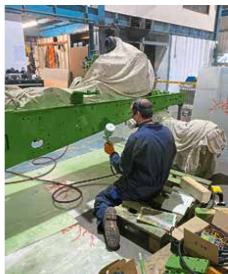
The engine, gearbox, axles and chassis were resprayed 'in-house', this also allowing various items to be repainted as appropriate as the rebuild progressed.
