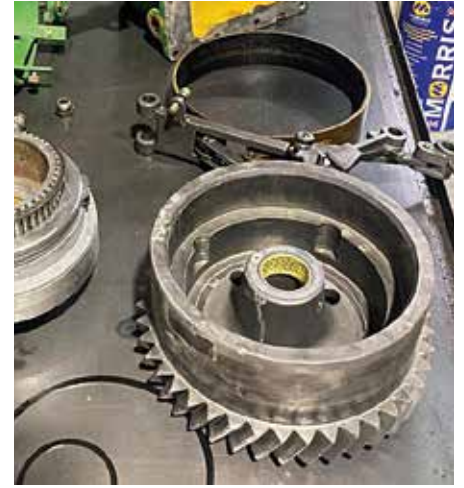
As part of the gearbox rebuild it was discovered the brake band had failed causing much of the damage within the transmission. Original 6000 series brake bands are no longer available but fortunately one from the newer 6030 series can be adapted to fit, with the added advantage of providing for a more robust repair. This is what is now nestling inside the fully refurbished gearbox.
