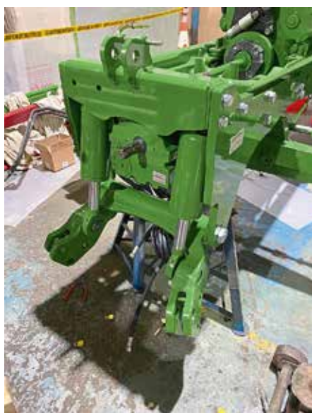
The front linkage mounting brackets bolt directly to the chassis of the tractor, with large lift rams ensuring the nominal 2.8 tonnes of lift is delivered swiftly. With around 100hp available at the pto, this set up will easily handle a 3.0m front mount mower.
