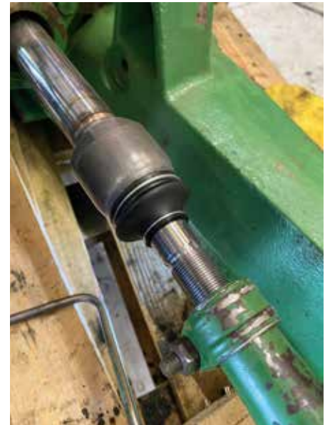
New track rod end boots, track rod adjuster joints and new pivot bearings were fitted to the front axle. Previously removed hubs filled with dirty black oil but no defects inside they were reassembled and will be colour matched with new wheel rims.
