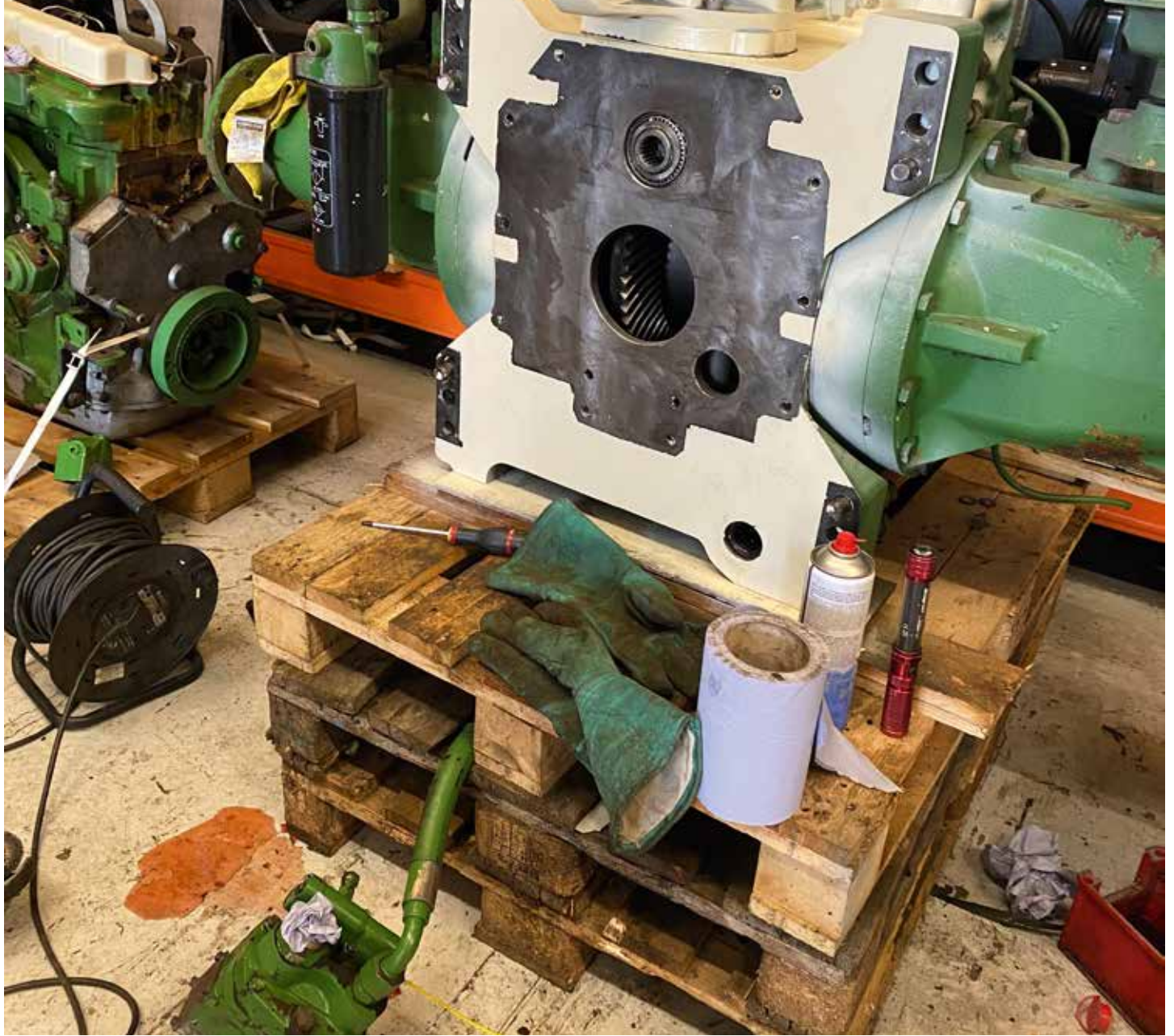
Once checked and re-assembled, the rear axle face was primed ready for paint with the joint surface masked off and cleaned for a leak free seal when refitted.
