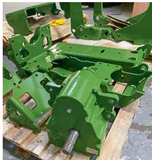
The Zuidberg front pto kit was added to complement the refurbished front linkage and benefits from a 'soft start' engagement system. Note the pick-up hitch hook mounted to one side, with space for the drawbar or ball hitch on the other.
