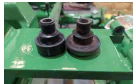
Greg Allen, a key member of the restoration team, has primed and painted all major and minor parts and installed new perishables, such as new mounts. Correct cap head chassis rail bolts have replaced hex head items, that were not of the correct hardness, and have been, like refitted bolts, torqued up as per the workshop manual. Attention to detail should ensure the finished tractor looks and 'feels' like it did when new.
