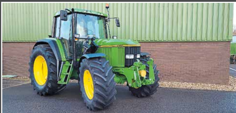
Fitted with taller and wider BKT 540/65 R28 and 650/65 R38 tyres, the completely refurbished Lynx John Deere 6800 certainly looks the part, particularly in comparison to how it arrived in October 2021. The original aim was to demonstrate how an aging tractor can be updated to match current demands, but the desire to get the tractor right saw the project take longer than planned. Next month we will look at some of the costs involved including fitting the various upgrades.
