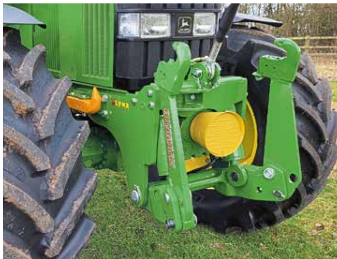
The Zuidberg front pto kit was added to complement the refurbished front linkage and benefits from a 'soft start' engagement system. Note the pick-up hitch hook mounted to one side, with space for the drawbar or ball hitch on the other.
