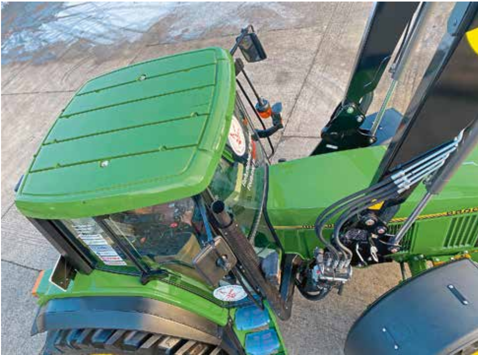
A solid roof, without hatch, is less common which in turn led to problems when it came to sourcing a new headliner for the cab. Note the amber beacon folded down beside the cab and the almost dainty exhaust stack. Visibility from the 6800 cab is excellent.
