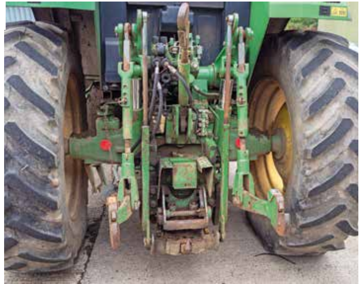
The Dromone rear pick-up hitch was well-worn and will be fully refurbished.
