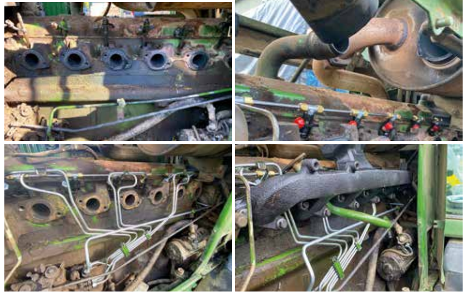
A rough running engine and poor starting was initially traced to the injectors. Their removal and replacement with refurbished items, plus new fuel lines, enabled the engine to be run and checked over, but this was just the beginning.
