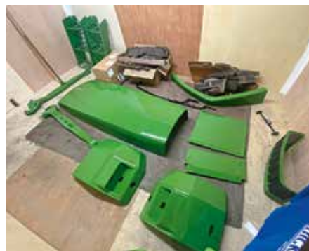
A 'dry room' was fabricated to house freshly painted parts to ensure they were protected up until the point of fitting. Easily lost or damaged components were also stored this way, taking pictures of removed bits and pieces where they were left helping locate them as the tractor was reassembled.
