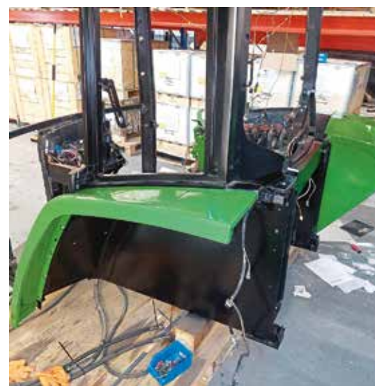
The cab was completely stripped, the frame receiving a fresh coat of black paint matched to the factory original.
