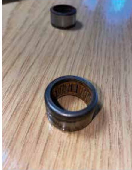
One of the pivot points for the auxiliary belt tensioner needed to be replaced, the pivot point having been eaten into by worn bearings. The rest of the system and bracket were sound. This wear is not repairable and is normally remedied by replacing with a complete tensioner kit. A local engineering firm made up a new pivot, and had it hardened. Once new bearings were sourced, the pivot was good as new. A full replacement kit would have cost in the region of £600 plus.
