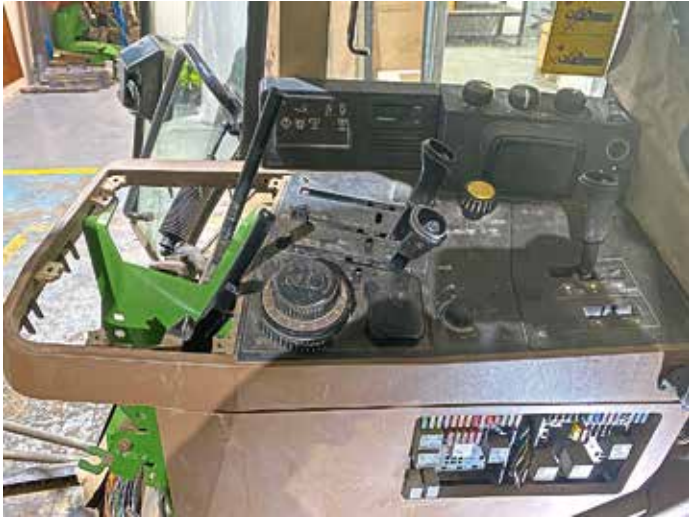
Notes of parts needed to refurbish the cab interior included sourcing new control lever caps from John Deere. Although the cab plastics were complete, a great deal of effort went into cleaning, strengthening and refinishing worn areas to give an 'as new' finish.
