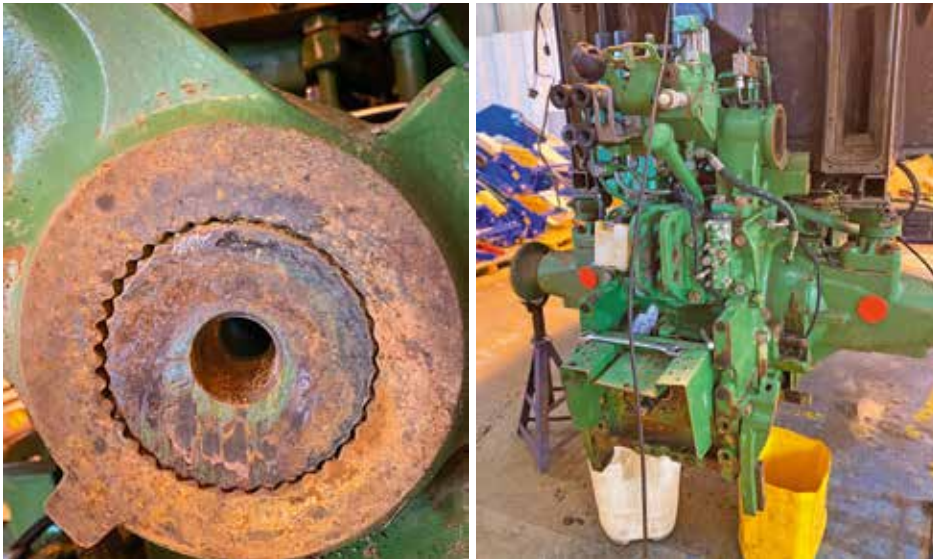
The cross shaft on the rear linkage shows wear typical of this generation of 6000 series, the back end of the tractor, prior to removal, otherwise presenting in good condition.
