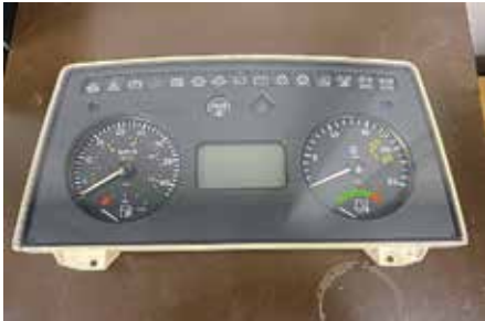
The dash binnacle was in good condition, with the instrument cluster responding well to a thorough clean. The scratched and faded Perspex was replaced and is now as clear as it was when new. The raised and white lighting and wiper symbols needed to be repainted, with certain areas of faded plastic being treated ahead of being airbrushed back to the correct colour. Restoring the areas the driver 'sees' was time consuming but just as important as getting the mechanical elements of the build right.
