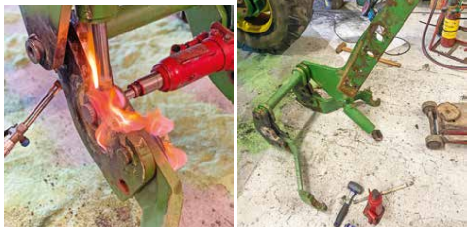
Thirty years of life on the farm saw numerous nuts, bolts and pivot points resist dismantling attempts, with heat facilitating the removal of the front linkage and its separate mounting frame. The linkage was in good condition but will be refurbished with new bushes and be joined by a freshly installed front pto with override system.
