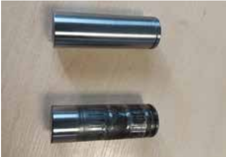
One of the pivot points for the auxiliary belt tensioner needed to be replaced, the pivot point having been eaten into by worn bearings. The rest of the system and bracket were sound. This wear is not repairable and is normally remedied by replacing with a complete tensioner kit. A local engineering firm made up a new pivot, and had it hardened. Once new bearings were sourced, the pivot was good as new. A full replacement kit would have cost in the region of £600 plus.
