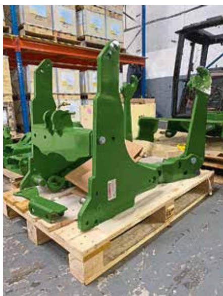
The front linkage mounting brackets bolt directly to the chassis of the tractor, with large lift rams ensuring the nominal 2.8 tonnes of lift is delivered swiftly. With around 100hp available at the pto, this set up will easily handle a 3.0m front mount mower.
