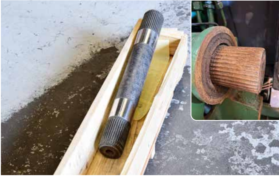
The cross/rocker shaft, that connects the upper arms of the three-point linkage, had severely worn splines (inset). A replacement part was listed as available from a pattern parts specialist for around £500, but after two months of waiting and still no sign the decision was made to purchase the genuine part which was in stock but with a significantly higher price tag.
