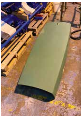
All painted metal, to include the bonnet, side panels, front fender mounts and rear mudguards, will be or have already been shot blasted and primed in a two-pack epoxy primer ahead of having a topcoat of JD green applied. Opting for a high-quality primer will ensure the new paint has high adhesion and will provide a good base for the colour coat. Talking of colour, John Deere green from the 1990s is a different shade to that currently in use. After asking for the paint RAL code from a friendly John Deere dealer, the team were informed that it the colour is just "John Deere Green". A colour match was taken from the inside of one of metal side panels of the tractor, a paint specialist then taking a scan. This will ensure the finish is correctly matched to the production colour applied to the tractor when new.
