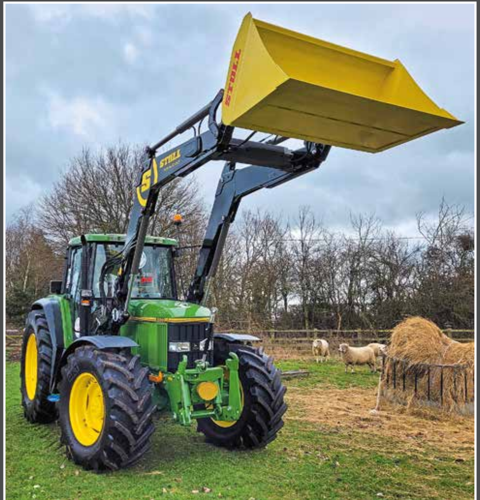
Back in 1992, the John Deere 6800 had a great deal to offer, its 120hp six-cylinder engine and 16-speed PowrQuad semi-powershift transmission remaining 'on the money' for many users today. Those seeking to press a refurbished model into front line use will have the benefit of readily available options to update the tractor.
