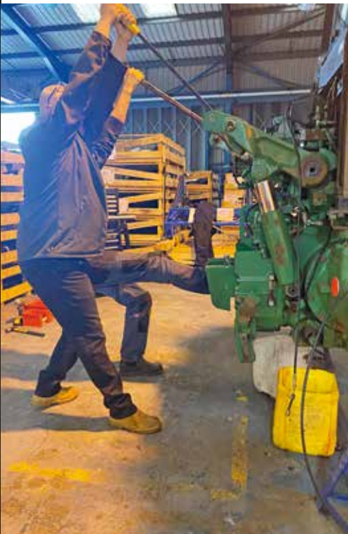
The back end required replacement of the main lift ram spigots due to a lot of wear. Luckily, they gave up with too much a fight and were removed without need for heat. The main lift rams are with a local hydraulics specialist for a rebuild to include new seals.
