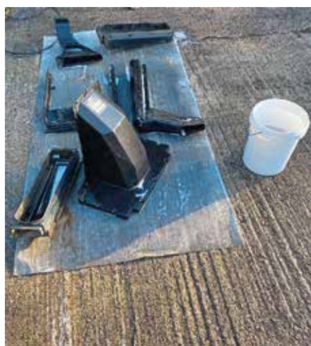
Moulded plastic parts are not easy to replace if damaged, with certain items needing to be repaired ahead of refitting. A great deal of time was invested in cleaning removed items, the quality of the original parts enabling them all to be reused on the finished tractor.
