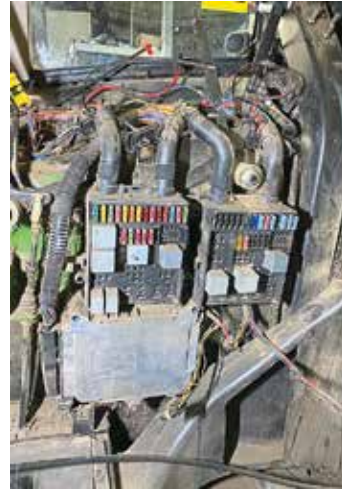
Although tractors made back in the 1990s have fewer electronics, that is not the same as suggesting the wiring looms are simple. Once internal cab cladding was removed, the amount of dirt found underneath reflected the tractor's hard life, all key connectors and fuses being covered ahead of a comprehensive clean.
