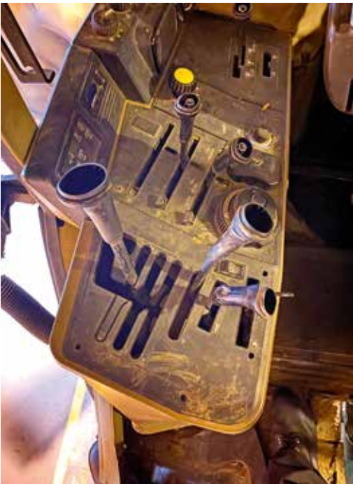
Popping off the lever knob end caps enables the nuts that hold them in place to be removed. The various knobs within the cab are in varied condition, a decision on what to renew being left until later in the project.
