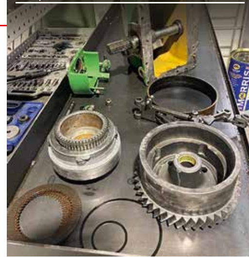
It was not until it was completely stripped and cleaned that the extent of the work needed on the transmission could be seen. From the clutch discs through to the brake band, new gearbox parts will cost in excess of £5,000.
