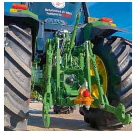
Completely refurbished to 'as new' condition, the rear linkage has quick couplers and a ball hitch fitted to bring it up to date.
