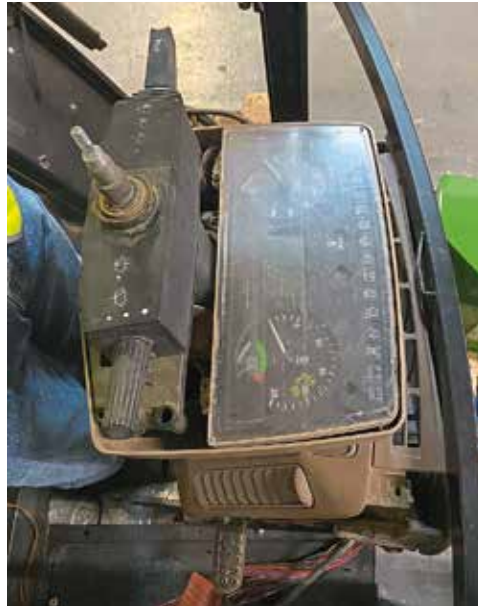
The dash binnacle was in good condition, with the instrument cluster responding well to a thorough clean. The scratched and faded Perspex was replaced and is now as clear as it was when new. The raised and white lighting and wiper symbols needed to be repainted, with certain areas of faded plastic being treated ahead of being airbrushed back to the correct colour. Restoring the areas the driver 'sees' was time consuming but just as important as getting the mechanical elements of the build right.
