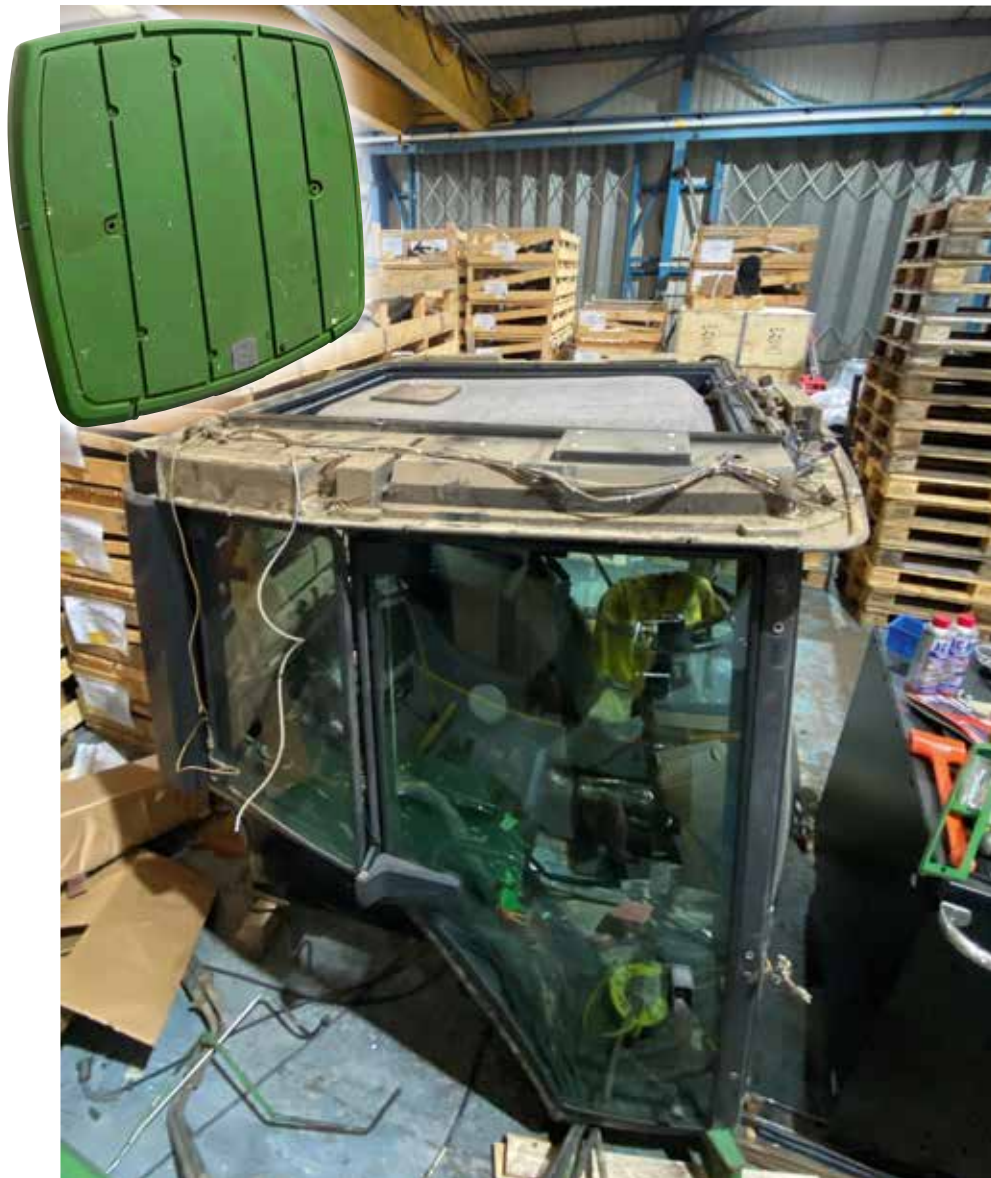
With the roof removed for painting, the sagging headlining was easier to get at but a new 'non-sunroof' replacement is no longer available. A fabric matched replacement will be sourced from either a UK or US based upholsterer and is yet another point that is holding up the build. Once all the sensitive parts and electrics are removed or covered, the cab will get a thorough clean.
