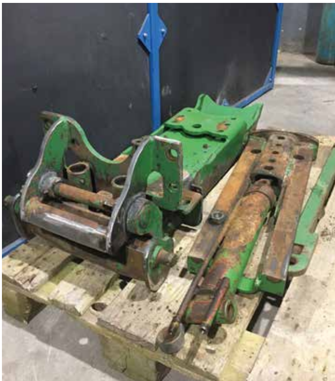
Refurbishing the original Dromone pick-up hitch is underway, this well-worn item needing a great deal of TLC to bring back to as new condition. The Flexxaire Fan will be measured up once the engine and radiator are installed.
