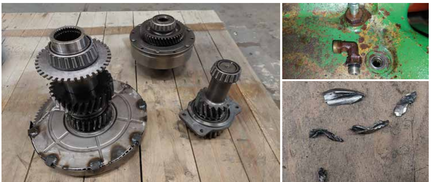
A rear axle leak needed to be sorted out, with one of the hose connectors on its last legs (middle). It was also found that there was an odd noise coming from the hydraulic pump when turned by hand. With the axle split, it was found the pump's oil guard had failed at some point but had been repaired (left). The guard cannot be purchased separately. Deere specialists at Cornthwaites suggested the guard could make a noise even when new, further examination showing the original repair had not included cleaning out swarf and fragments (right). Although scruffy, the existing weld repairs were sound and the gears were in decent condition so the the axle was reassembled and the halves re-joined using Loctite 574.
