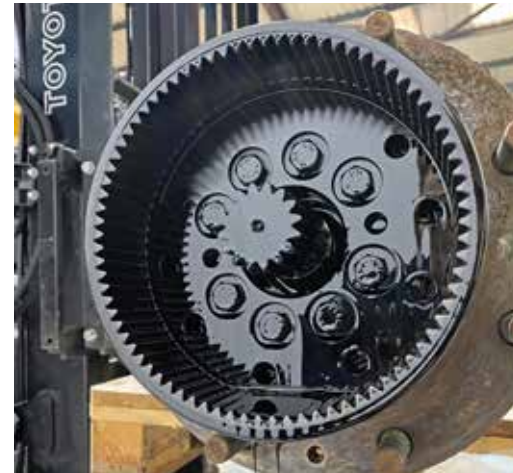
The oil in the front axle had not breached the hub seals, its black colour suggesting a lack of leaks also meant it was not checked or changed in a long time.
