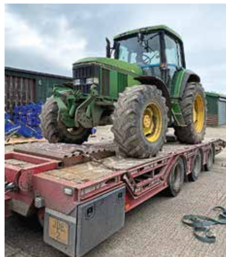
On arrival back in late 2021, the 6800 was fitted with 16.9 R24 and 18.4 R38 (metric equivalent 420/85 R24 and 480/85 R38) tyres. Fitting larger tyres transforms the overall look of the tractor, but other changes have also been made to bring the tractor up to date.
