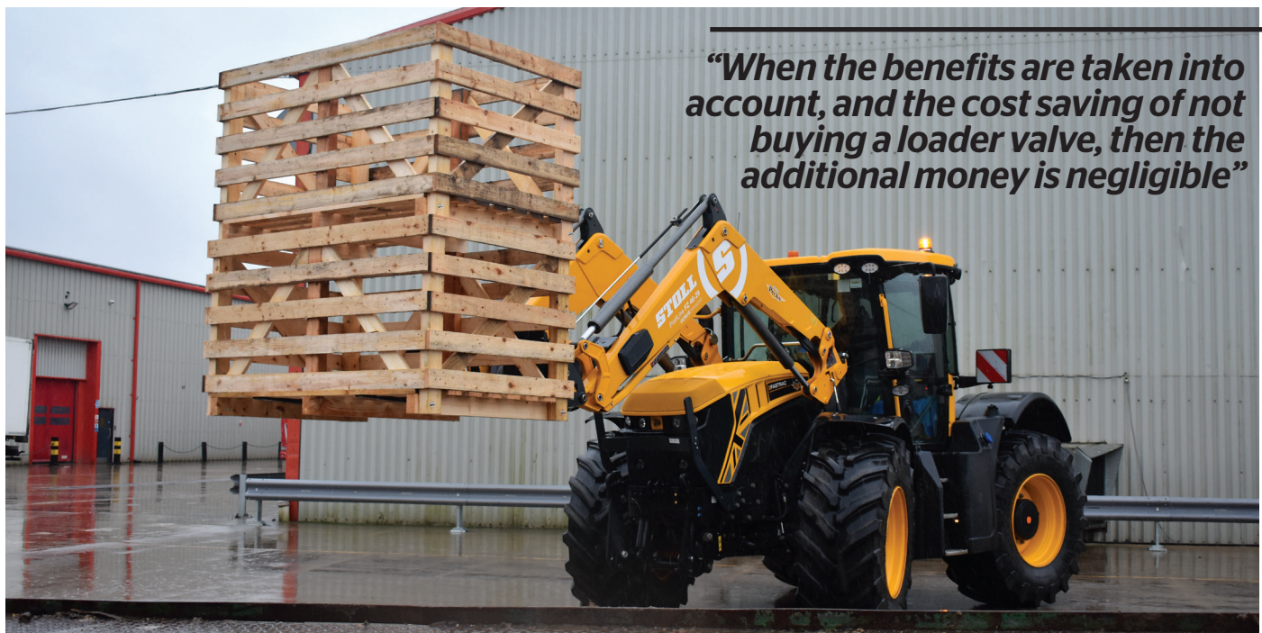
Above: Thanks to its self-levelling hydropneumatic suspension, JCB's Fastrac doesn't need a counterweight when used with a loader.
