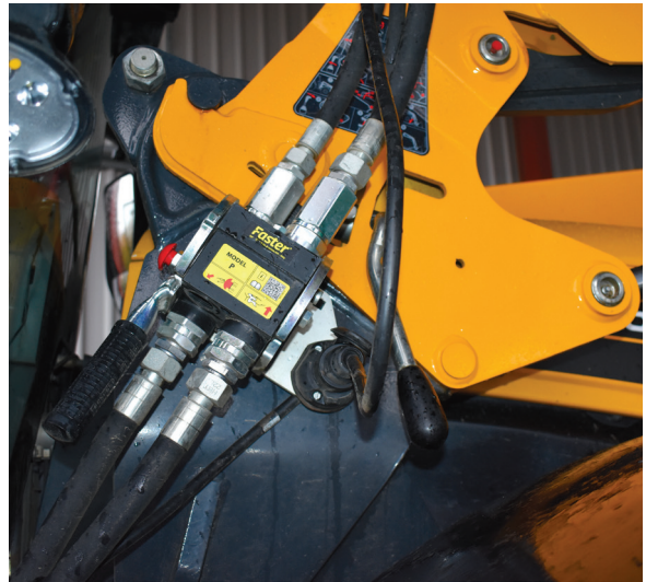
Above: A newly designed ISOBUS-compatible spool block is mounted on the loader crossbeam under this grey panel.
