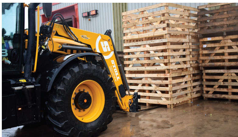
Above: Thanks to its self-levelling hydropneumatic suspension, JCB's Fastrac doesn't need a counterweight when used with a loader.
